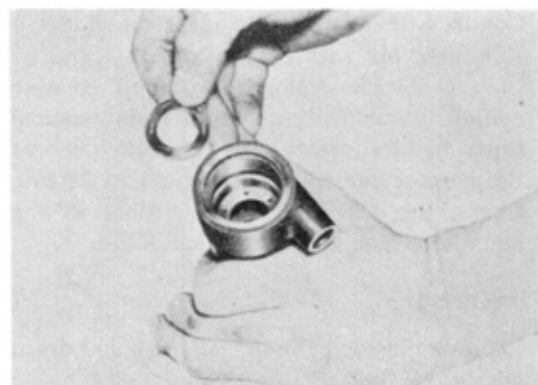
Fig. 1-25 Inserting Piston Cup Spacer & Piston Cup
